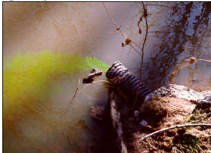
Figure 15: Dye at outfall location
